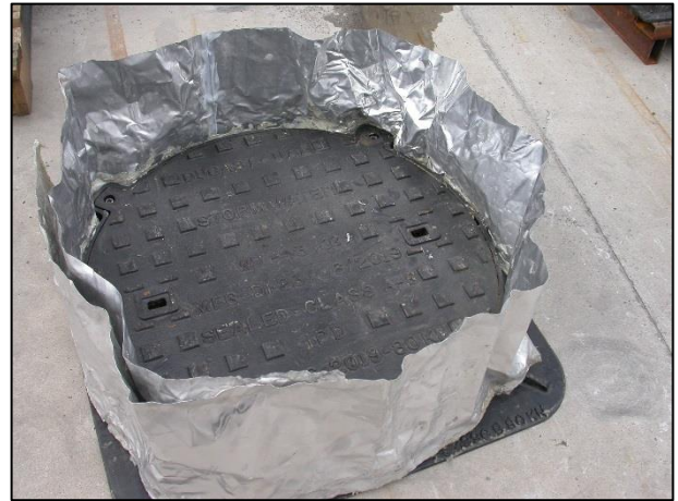
Figure: 4 Subject: Test set up for water/gas tightness
