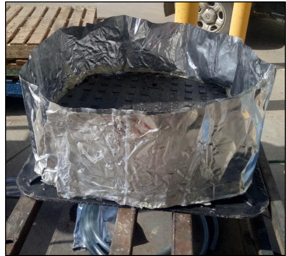
Figure: 4 Subject: Test set up for water/gas tightness
