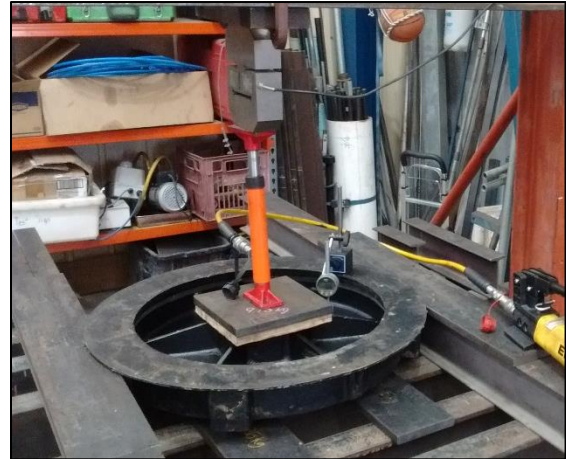
Figure: 4 Subject: Test set up for water/gas tightness
