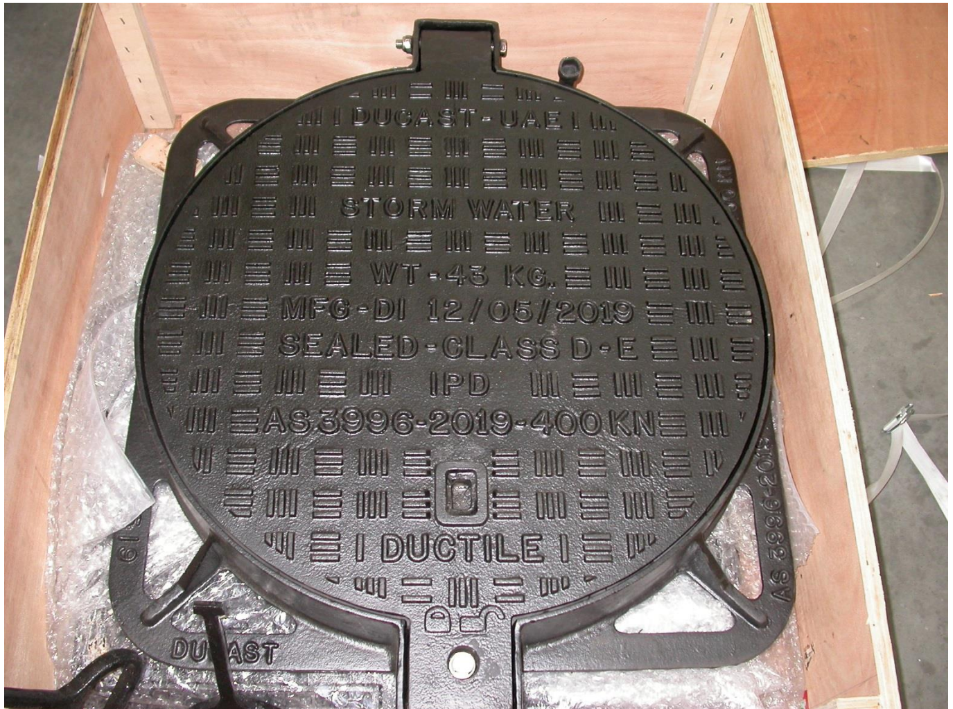
Figure: 1 Subject: Cover submitted for testing (note the hinge at the top end and securing bolts at the bottom)
