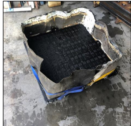
Figure: 4 Subject: Test set up for water/gas tightness
