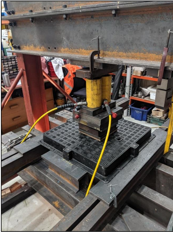
Figure: 5 Subject: Cover load test
